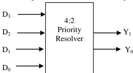
Fig3a: Block diagram of priority resolver
